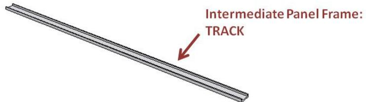
Design Considerations include: track span, track material, track thickness, connection of track to building frame.
