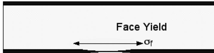
Figure 14 – Yielding of the Face (Tension)<sup>18</sup>
