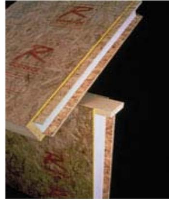
*A common SIP is comprised of interior and exterior OSB sheathing with expanded polystyrene core in the middle. CSIPs replace the OSB sheathing with cementitious panel such as Hardieboard.*
